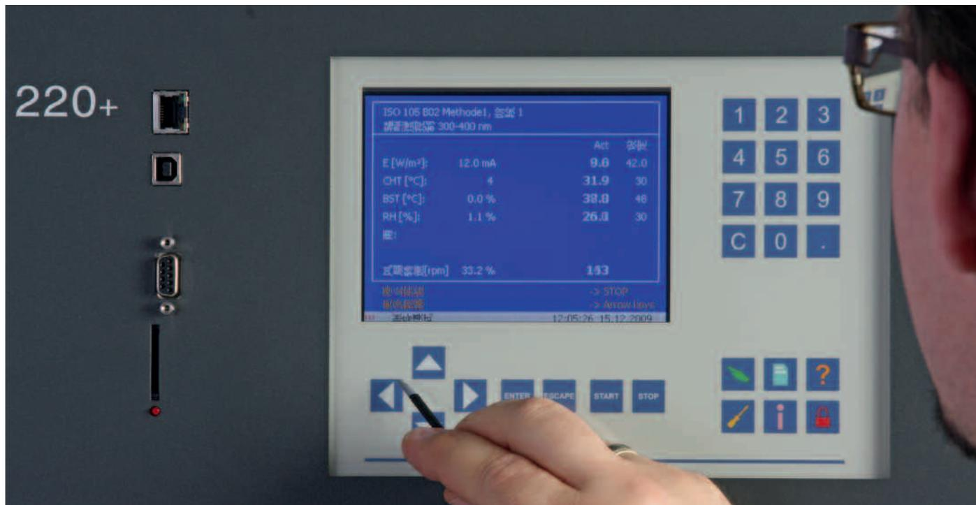
The **Xenotest® 220** and **220+** are digitally controlled. The touch screen and keypad control are both available in multiple languages, which enable easier handling after initial installation.
